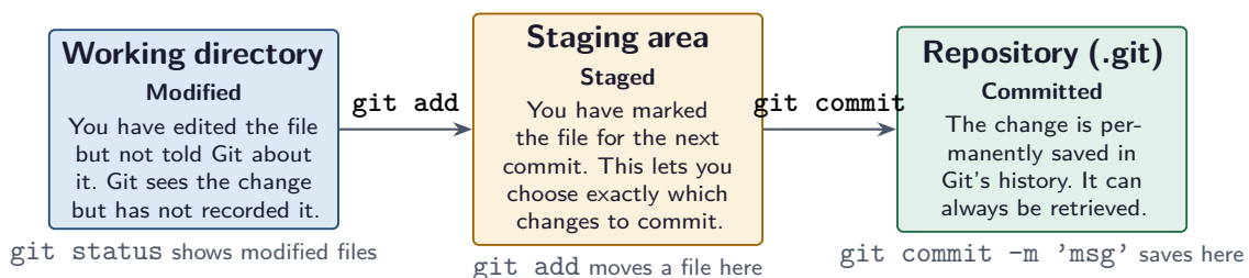
Figure 8.5: The three stages of a file in Git.
